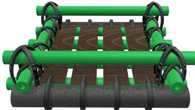
Figure 7: An example of how the floaters can be fastened on the frame using joined zip ties. While fastening the floaters you can fasten as well the wooden floor to the pvc frame.
