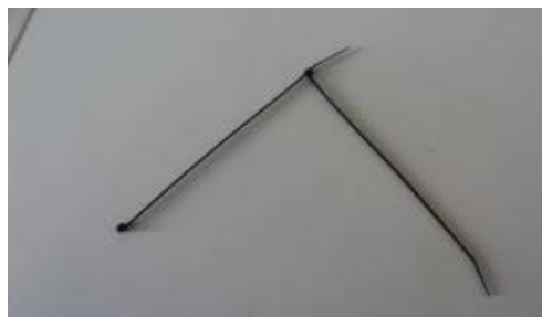
Figure 4: Two joined zip ties. In this way we can join together more than two zip ties in order to maximize the length.
