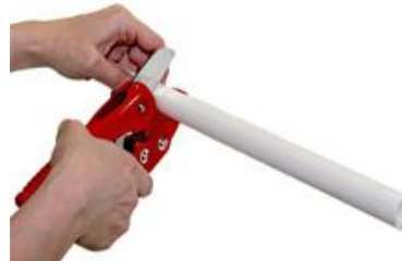
Figure 9. How to cut a PVC pipe
