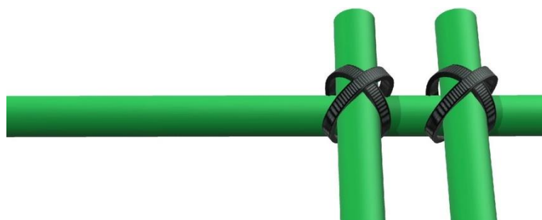
Figure 2: In this picture we can see how we can keep on fastening pipes together in order to construct the frame of the platform.
