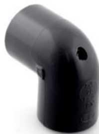
Figure 5. Drain hole drilled in a PVC elbow
