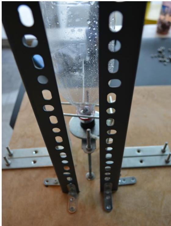
Figure 24. Two out of four Dexion angles attached to the wood base.
