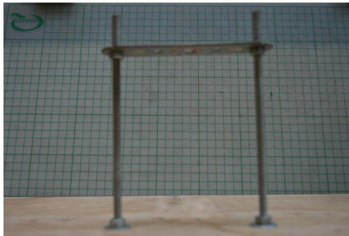
Figure 14. Nuts and mending plate attached to the threaded rods
