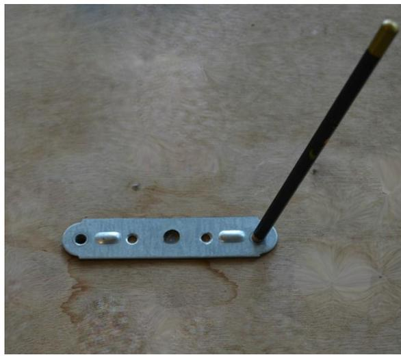
Figure 9. Mending plate on wooden base. Holes are marked using a pencil.
