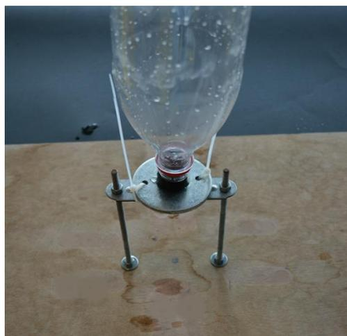
Figure 18. Bottle placed over the rubber stopper
